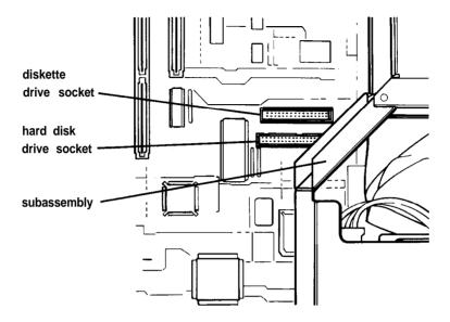
Both sockets have a notch on one side. The hard disk drive socket is a bit longer than the diskette drive socket.
